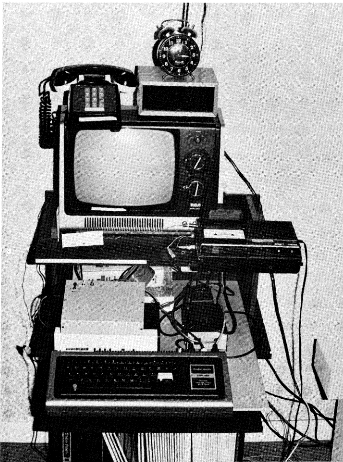
The author's system. The TV is driven by an RF modulator enclosed in the case that contains the Electronic Systems TRS-80 I/O board and power supply. This case is located just behind the keyboard on top of the A 103 modem.
